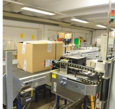
Other, so-called twin-tamp swivel applicators, are capable of labelling the front and top of passing products without stopping the products. It is even possible to dispense labels onto the inside of pipes or tubes or also "around corners" at varying length ratios, for instance, to allow reading information from two sides.
